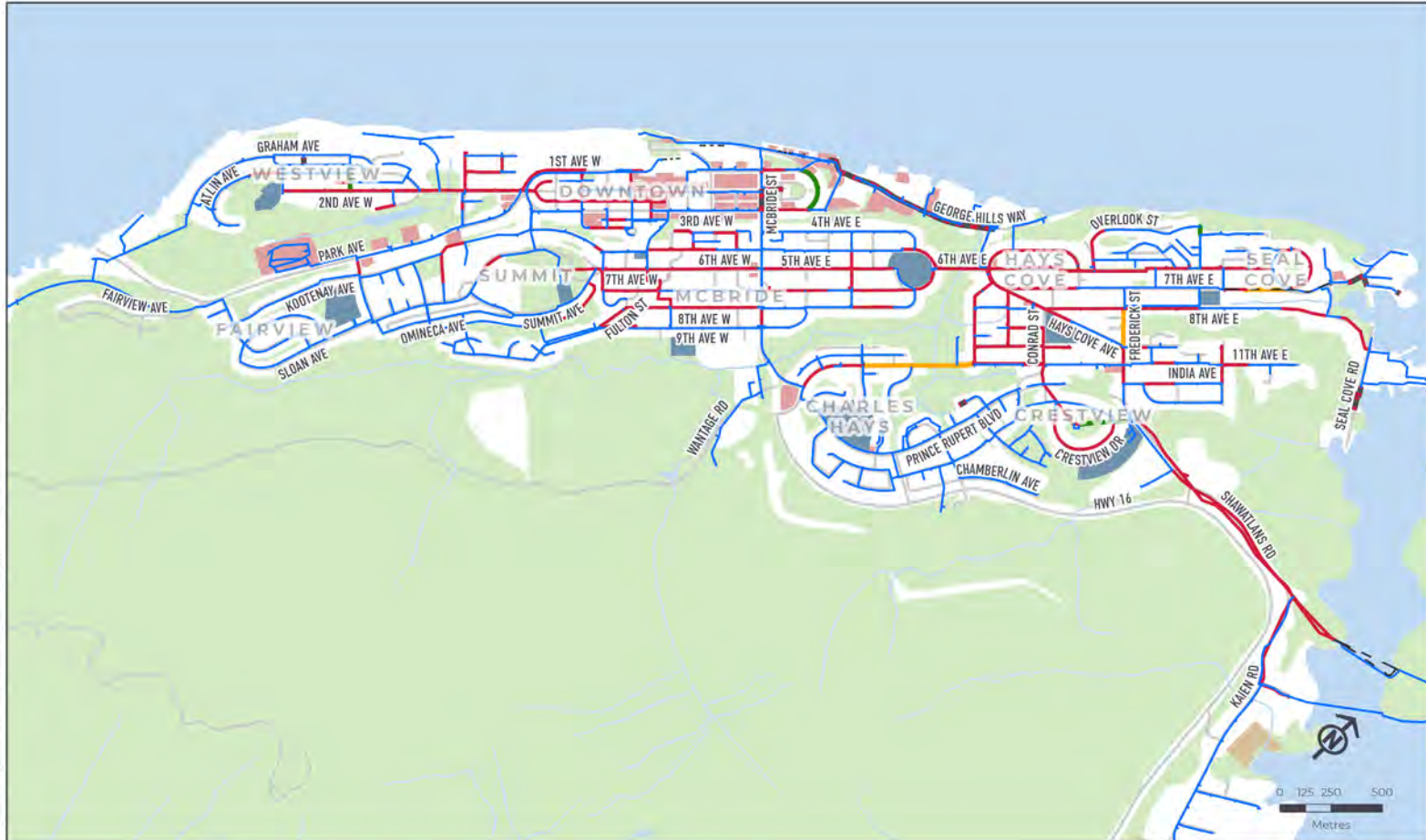
FIGURE 2 INFRASTRUCTURE REPLACEMENT PRIORITY
