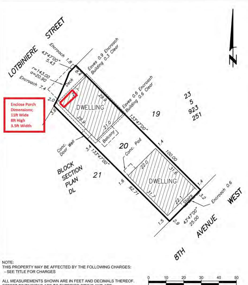
OFFSET DIMENSIONS ARE TO EXTERIOR SIDING AND ARE PERPENDICULAR TO PROPERTY LINES, UNLESS OTHERWISE SHOWN.
